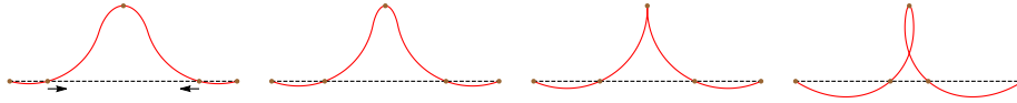
Figure 9: The creation of a cusp using clamped min eccentricity weights. Moving the 2^{nd} and 4^{th} points closer creates a cusp at an input point.
