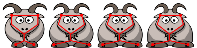
Figure 12: From left to right: the initial shape/control polyline and our deformed shape with c_i=1 and \beta = 1, 1.5, and 2 .
